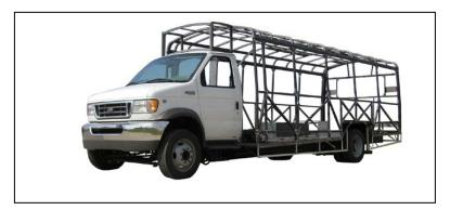
• Bus Bodies are square, level and plumbed prior to installation on the chassis. Other manufacturers attach their bodies to the chassis without using this methodology.
